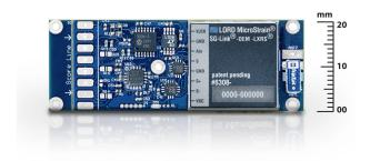
SG-Link<sup>®</sup>-OEM-LXRS<sup>®</sup> - small, low-cost two-channel analog sensor node ready for OEM integration
