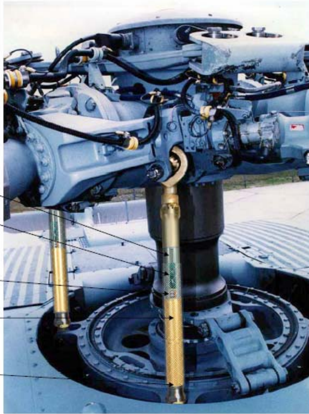
Figure 5. Graphic illustration showing wireless load sensing pitch links with energy harvesting, energy storage, data processing, and RF communications elements.
