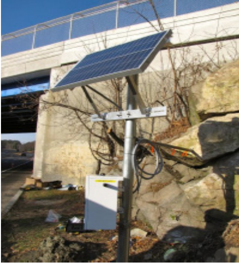
WSDA-1000 Wireless Sensor Data Aggregator in an environmental enclosure, with solar array.
