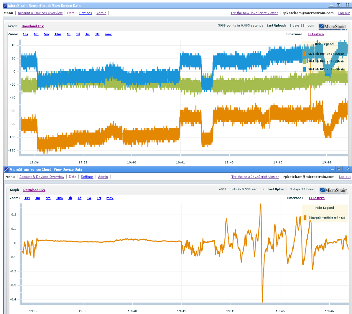
Figure 11. Flight test data - Wireless Strain (top) vs. Vehicle Yaw sensors (bottom).
